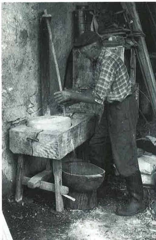
Fig. 12. Grinding with hand-mill equipped with wooden axle. Mogyoróska, North Hungary, 1976.
